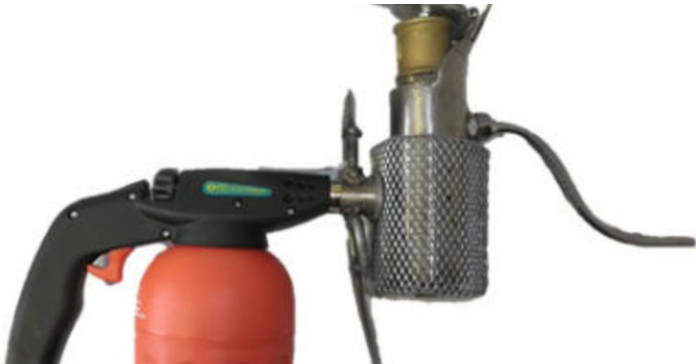
Machine for oxalic acid application
