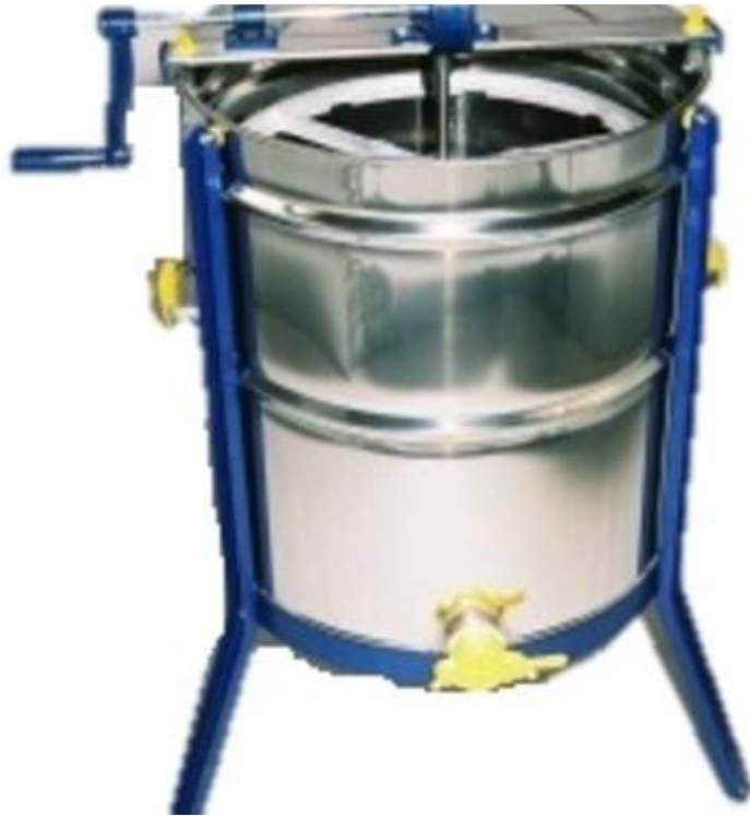
Stainless steel manual radial extractor 12 frames ½ handle
